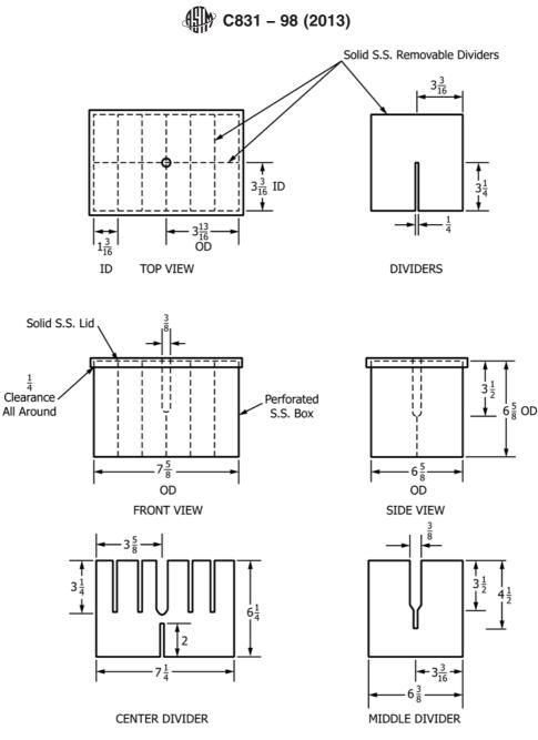
NOTE 1—Type 316 stainless steel (S.S.) or other suitable alloy, 14 gage (1.984 mm). Perforated S.S.: 14 gage. <sup>3</sup>/<sub>16</sub>-in. (5-mm) diameter perforations, <sup>1</sup>/<sub>2</sub>-in. (13-mm) centers, 11% open. Note 2—Dimensions are in inches.
