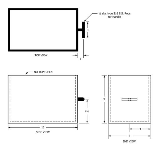
NOTE 1—Material specified is type 316 stainless steel (S.S.) or other suitable alloy (¼ in. (6 mm) recommended). NOTE 2—All dimensions minimum outside diameter.
